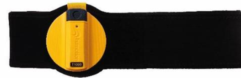
Make sure the black cap points upwards, and the sensor is aligned with the spine.
