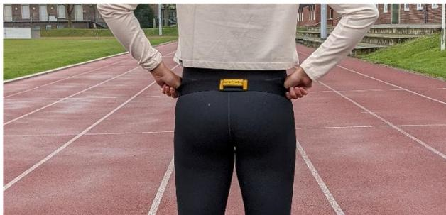
*The TB40 Belt is positioned on the lower back with the DX5.0 sensor aligned with the spine. The black sensor cap points to the left and the Humotion logo on the sensor faces outwards.*
