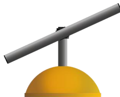
Figure 3: Angled magnetic element (Cone + angled mount + magnetic rod (MCD))
